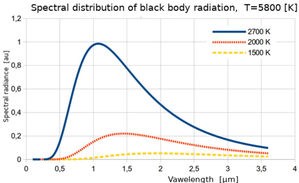
Figure 2: Distribution of radiation power as a function of wavelength for different temperatures.
