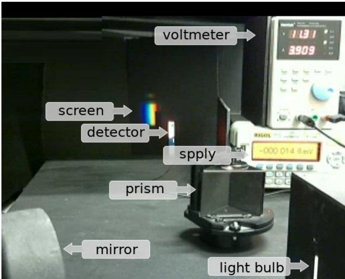
Fig. 4: A photo of the measurement system.
