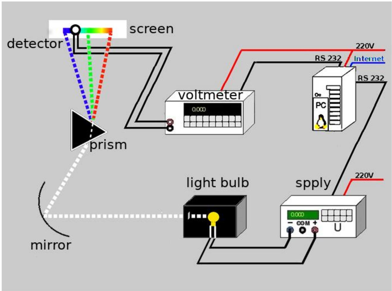
Figure 3: Diagram of the system for measuring the power of electromagnetic radiation.
