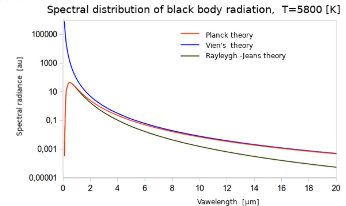
Figure 1: Comparison of Wien's, Rayleigh-Jeans' and Planck's theories for distribution of radiation power as a function of radiation wavelength.
