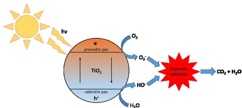
Figure 4: The mechanism of photocatalysis.
