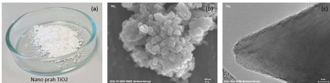
Figure 1:  $\text{TiO}_2$  nanopowder. (a)  $\text{TiO}_2$  as seen by the naked eye, (b) a cluster of  $\text{TiO}_2$  particles and (c) a single  $\text{TiO}_2$  particle as seen using electron microscopy.
