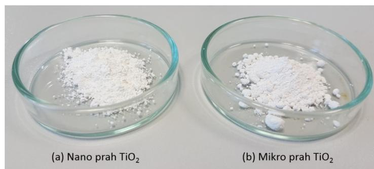
Figure 2:  $\text{TiO}_2$  nanopowder and  $\text{TiO}_2$  micropowder.
