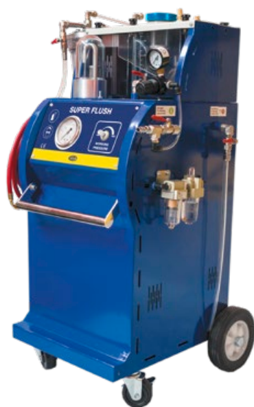
007936211000 Device filter Super Flush with microfiber
