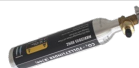
CO2 refrigerant cylinder for MB 007950027565 Refrigerant weight: 340 grams/ empty cylinder: 926 grams
