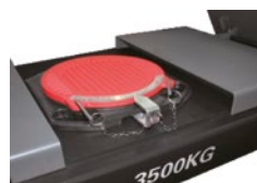
Turntables and rear suspension release plates
